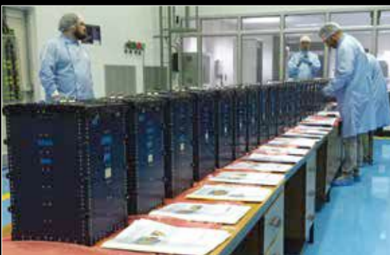
The array of 25 Quadpack Dispensers, protecting the 96 Nanosatellites placed within it
