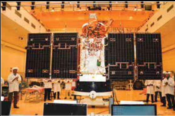
Cartosat-2D undergoing Solar Panel Deployment Test
